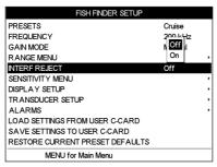
Figure 17.9 - Interference Rejection menu
